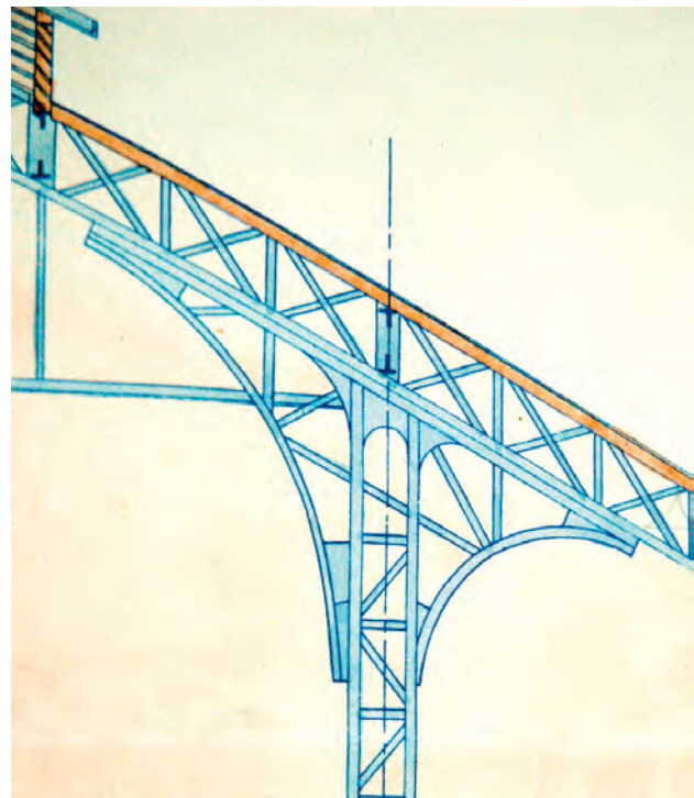
Fig. 29. Detail of the pillar supporting the slanted beams of the roofing. All the constructive elements have composite sections made of laminated profiles (AN-DMB, PMB, Technical Service, File 28/1893, f. 135).
